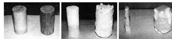
Xypex-treated mortar and untreated mortar were measured for acid resistance after exposure to a 5% H<sub>2</sub>SO<sub>4</sub> solution for 100 days. Xypex suppressed concrete erosion to 1/8 of the reference samples.
