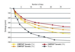
Tests on ISO mortars at 20°C, 50% HR
